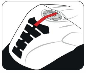
2. Use a piece of tape to hold protector in place central to the tank
