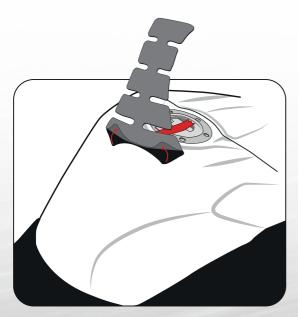
3. Lift protector and peel the top corners of protective film.
