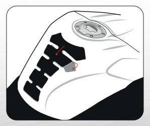
4. Remove the tape. From top to bottom slowly peel the remainder of the protective film away, pushing the protector in to place as you go.
