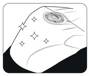
1. Clean tank with lint free cloth to remove grease and dirt
