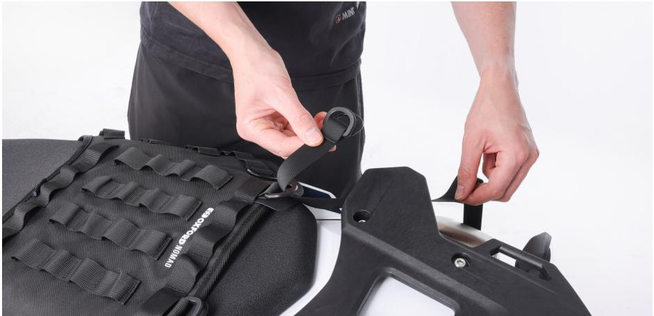
4. Find a location to secure the D-ring straps (**B**) around the motorcycle frame so that it does not interfere with the chain, foot pegs or foot levers.
